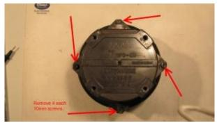
Step 3: Flip the rotor over and using a 10mm wrench remove the 4 screws holding the bottom bearing race to the moving bell.
