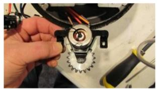
**Step 9:** Notice the 4 wires connected to the pot.
